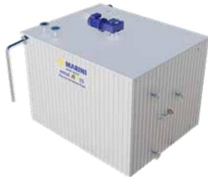
emulFALT's **water-acid-emulsifier preparation tank's** body and heating coil pipes are constructed with **316L stainless steel** and tank is **covered with rockwool insulation**. No.1, 3kW, direct coupled with a gear-motor agitator with 316L stainless steel shaft and blades, equipped with protected bearing housing at the bottom of the tank.
