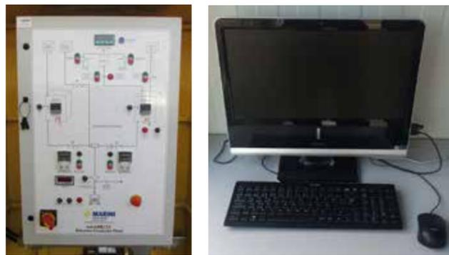
Control system of the emulFALT is **manual as a standard**. However, PLC & SCADA control system with embedded touch screen computer on the control panel or control cabin with PC options are available.
