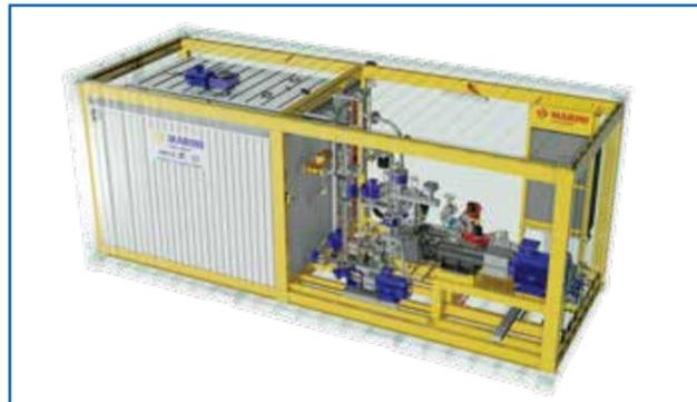
emulFALT15 emulsion plant is designed as a compact machine in order to be transported by 20' OT container, especially for overseas trades.
