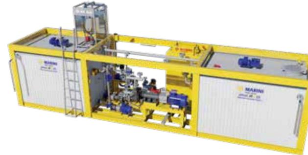
Integrated Bitumen Tank (IBT) with 9 ton capacity is a perfect solution to keep small amounts of bitumen at required temperature without heating up/cooling down the whole bitumen storage to operational values; and therefore, reducing heating costs. Additionally, it provides production flexibility by allowing to add & mix (with agitator) solid and liquid additives directly into the bitumen prior to milling process.
