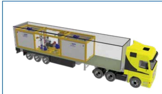
Integrated Bitumen Tank (IBT) option is a flexible solution for different emulsion applications. emulFALT15 with IBT can be transported easily by a truck and also 40' OT container all around the world.
