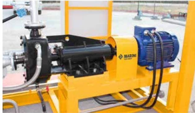
emulFALT's **emulMILL** with its **adjustable milling gap** provides <math><6\ \mu\text{m}</math> particle size and guarantees the best quality of final product even with low penetration bitumen. Thermal oil or electrically heated mill is suitable for the production of both anionic and cationic emulsions and also modified bitumen emulsions.
