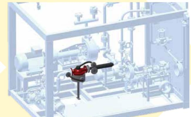
Bitumen mass flowmeter to produce high-quality emulsion. Thanks to bitumen flowmeter; the actual amount of bitumen flow, total amount and other parameters can be checked and adjusted properly.
