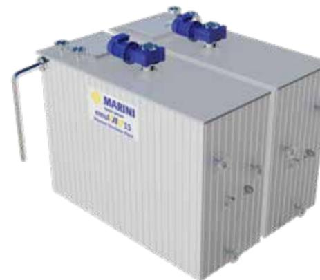
The integration of Twin WAE Tanks reduces the batch intervals, thus capacity increases with continuous production. While WAE mix is being prepared in one part of the tank, ready WAE mix is being fed into the system.
