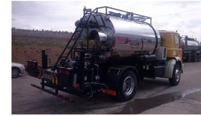
It has proven itself with many advantages and production flexibility that it provides to users. With automatic spraying, it sprays the optimum amount of material and also saves heating costs thanks to its insulated body.
